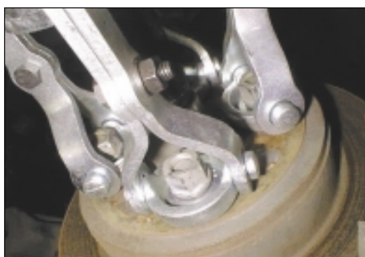
a) Hydraulic ram c) Pulling arm
