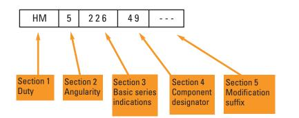
A new inch part numbering system was developed by the American Bearing Manufacturers Association (ABMA) to address the expansion in the number of new applications and tapered roller bearing designs. This part numbering system has become the international standard for inch-sized bearings.
